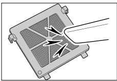
Remove dust from the filter using a vacuum cleaner or dry cloth.
